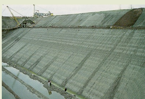
Figure 19 – Overview of a clay quarry (Kruibeke) showing the characteristic band structure of Boom Clay.
