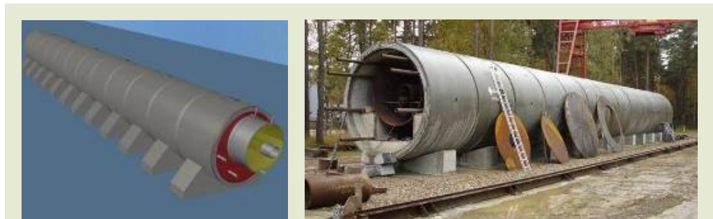
Figure 67 – Full-scale mock-up of a disposal gallery (with diameter 3 metres, length 30 metres and built-in simulation of heat-generating waste) developed, as part of the ESDRED Project, to demonstrate the feasibility of repository backfilling.
